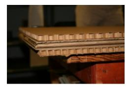
For small objects, several layers of sturdy cardboard may be used in lieu of honeycomb board. The cardboard must be rigid and dense enough to resist puncturing or bending. If layers of corrugated board are used, place each sheet with the grain perpendicular to that of adjoining layers for increased rigidity.
