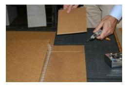
After retracting your blade, score the two remaining pencil/pen lines so that you can fold the remaining wings of the board upward. Include the small flaps as well (gently, so as not to tear them).
