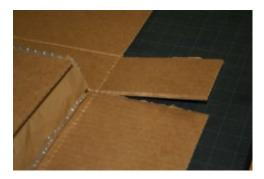
Fold the two long sides (with the smaller flaps) over the inner package and fold the small flaps in around the corners of the inner
