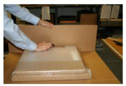
Make a second score line parallel to the first on each "wing" along the top edge of the inner package and continue to the outer edges of the board again so you can then fold the wing downward on top of the package.
